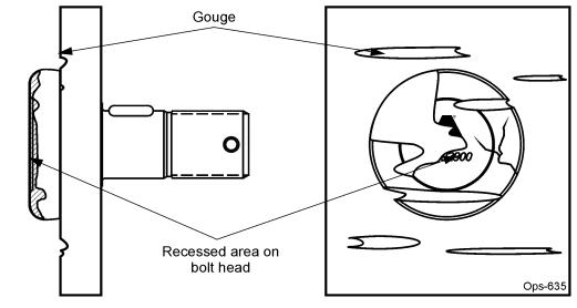
Inspect the Blade Bolt Heads daily for abnormal wear. REPLACE BOTH BLADE BOLTS on the Blades IMMEDIATELY if either blade bolts has:
